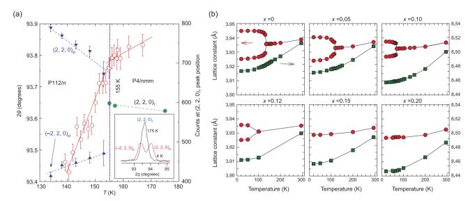
Figure 2. (a) Neutron scattering result on structural transitions on LaOFeAs [58]. (b) The temperature dependence of lattice constants for different F-doping levels in the SmFeAsO<sub>1-x</sub>F<sub>x</sub> system.
