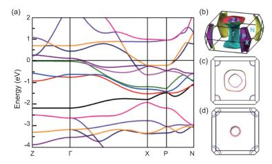
**Figure 14.** (a) Electronic band structure and (b) band structure in the PM phase for  $BaFe_2As_2$  in the folded Brillouin zone. (c) and (d) are the sectional views of the Fermi surface through symmetrical k-points Z and  $\Gamma$  perpendicular to the z-axis, respectively [193].
