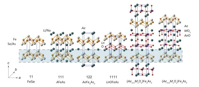
**Figure 1.** The schematic view of the crystal structures for several typical types of iron-based superconductors, in which A, Ae, Ln, and M stand for alkali, alkali-earth, lanthanide, and transition metal atoms.
