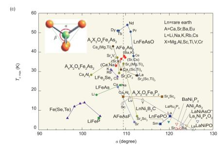
**Figure 4.** (a) Anion height dependence of  $T_c$  in iron-based superconductors [63]. (b) Anion height dependence of  $T_c$  in FeSe-derived superconductors [36]. (c) The relation between the As(top)-Fe-As(top) angle  $\alpha$  and  $T_c$  of iron-based superconductors [64].
